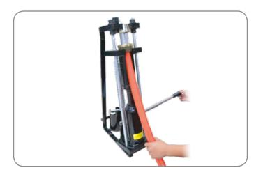
Insert coupling completely into the pusher. Using jack handle advance cylinder upward. As fitting approaches die opening properly align for entry of the coupling by deflecting the hose as required. Exert an upward force to ensure fitting is completely inserted into the pusher.
