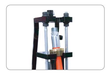
Remove or elevate one die segment to allow installation of the hose and coupling.
